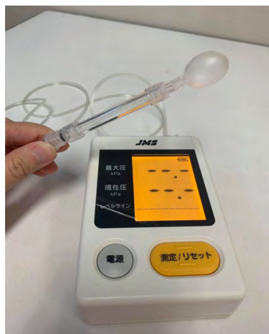
Figure 1 JMS tongue pressure measurement device (Orarize ® TPM-01, JMS Co.,Ltd. Hiroshima, Japan)
