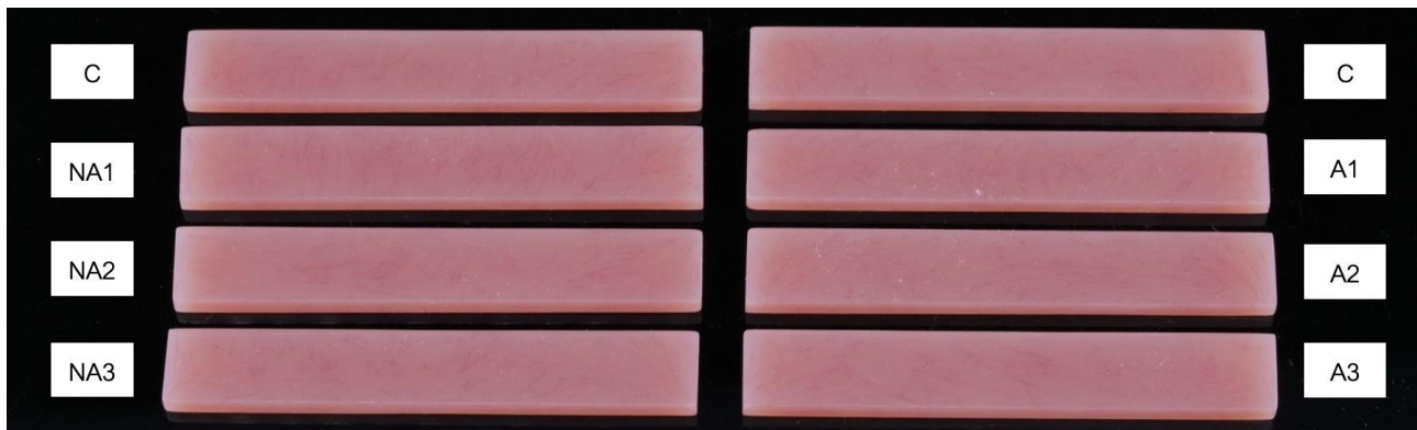
Figure 2 Polished heat-polymerized acrylic resin specimen of each group (65*10*3 mm 3 )
