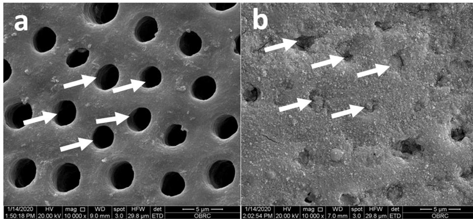
**Figure 2** Representative SEM micrograph of dentinal tubule (a) after immerse in 1% citric acid and (b) after brushing with Sensodyne Repair & Protect<sup>®</sup> 10,000 cycles with V-8 cross brushing machine (Sabri Dental Enterprise, Inc., USA) (b) (10000x magnification)
