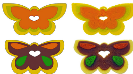
a) Multiple material cookies 3D model b) Actual printed cookies
