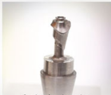
Customized contour milled by CAD-CAM system
