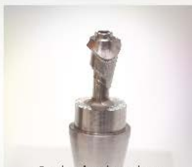
Customized contour milled by CAD-CAM system
